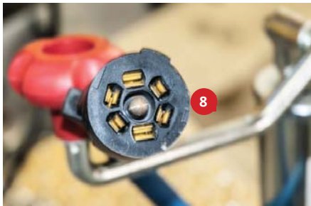
Trailer Electrical Hook-Up (6 Rounds)
