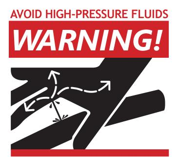
Escaping fluid under pressure can penetrate the skin, causing serious injury. Relieve pressure before disconnecting hydraulic or other lines. Tighten all connections before applying pressure. Keep hands and body away from pinholes and nozzles which eject fluids under high pressure. Use a piece of cardboard or paper to search for leaks.
