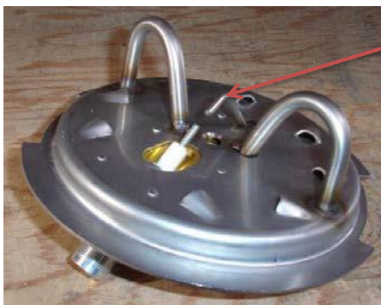
Figure 5-4 Igniter Plug Adjustment Point
