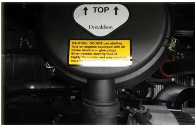
Air cleaner and filter assembly located
