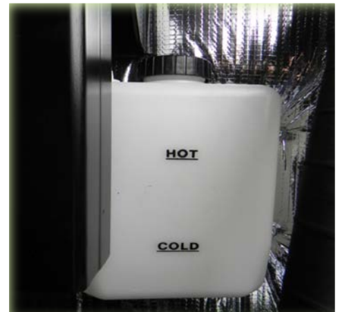
Heating fluid overflow (LRF) accessible from the right side of unit. Open front door and overflow is located to the right on the back wall of the unit.
